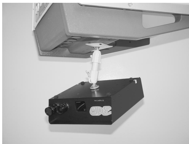
FIG. 1. The RealScan 3-D Laser range scanner mounted to an OR mechanical arm.
