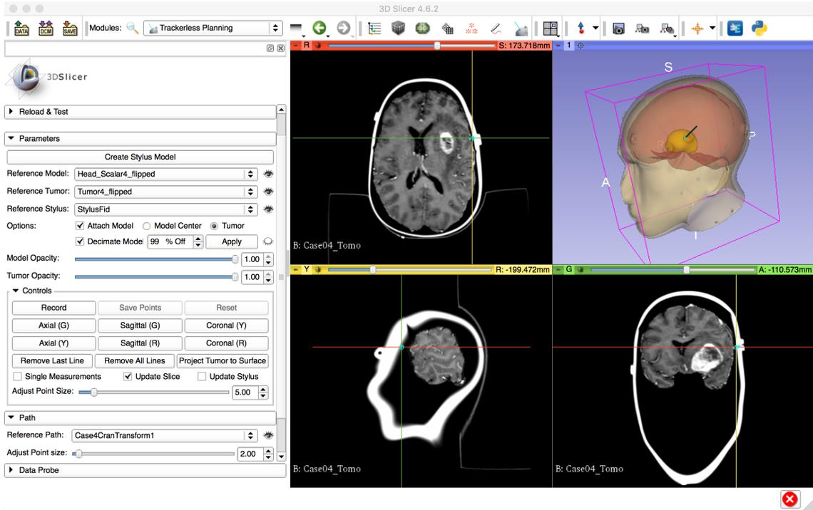
Figure 1. Overview of the trackerless surgical planning extension. Virtual stylus and traditional three-panel display allow simulation of conventional approach.
