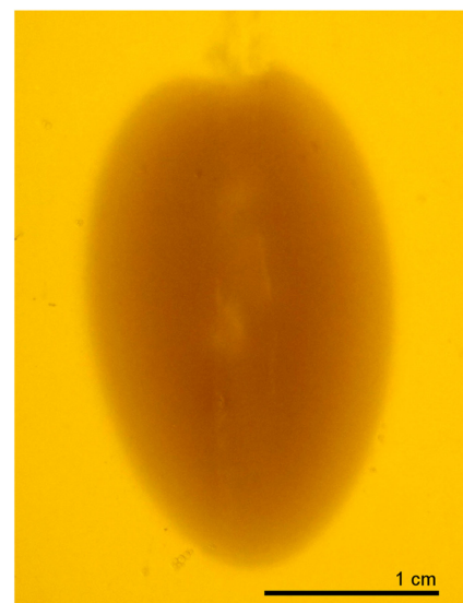
Fig. 2. Sample mock gross pathology of ablation zone (cut along the axis of the Perseon ST antenna) following an ablation at 60 W for 15 minutes in an agar-albumin phantom.
