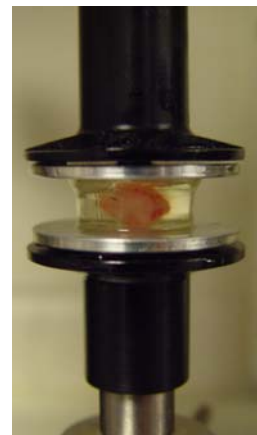
Figure 2. Example of a gel-tissue sample in the mechanical testing setup.
