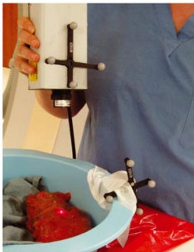
Figure 5. Conoscopic surface measurement of a human *ex vivo* kidney covered in perirenal fat
