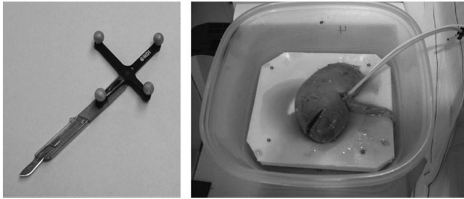
FIG. 1. Container and tracked scalpel for porcine kidney incision. Left: scalpel with Polaris target attached to handle, used to track an incision made to the renal parenchyma. Right: porcine kidney with glass bead fiducials attached to the surface to track deformation. The kidney was perfused with saline and cut with tracked scalpel.
