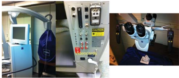
Figure 2: The Pentero microscope as a test-bed. (Left) Microscope, (middle) the two FireWire videocards for acquisition and (right) the head of the microscope.
