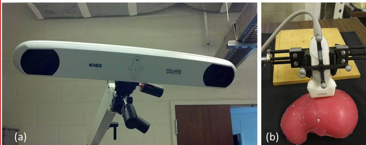
Figure 1. The tracked ultrasound system consisted of a Polaris optical tracking system (a) and a passive target attached to the ultrasound probe (b).
