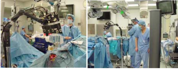
Fig. 1. (Left) LRS performing a scan during surgery. (Right) Scanner mounted on arm being tracked by the camera on right.
